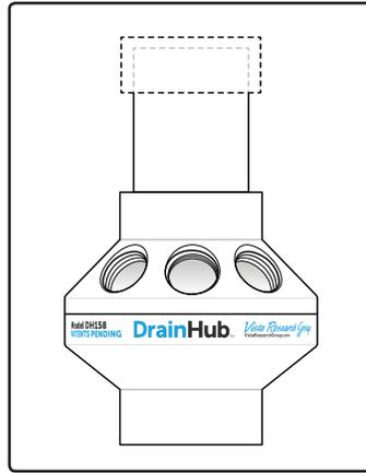
1-1/2" Pipe or Tube Stack (Open or Capped)
