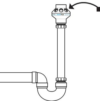
**Use DrainHub on a standpipe to connect:**
